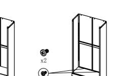
5. Install o into body of cabinet, as shown in the following figure
