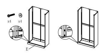
3. Install F into body of cabinet fix by screws
