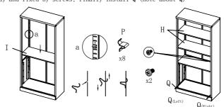
5. Place the assembled drawer attached to the cabinet, and adjust the spacing between the drawer and tighten  $\ensuremath{R}$
